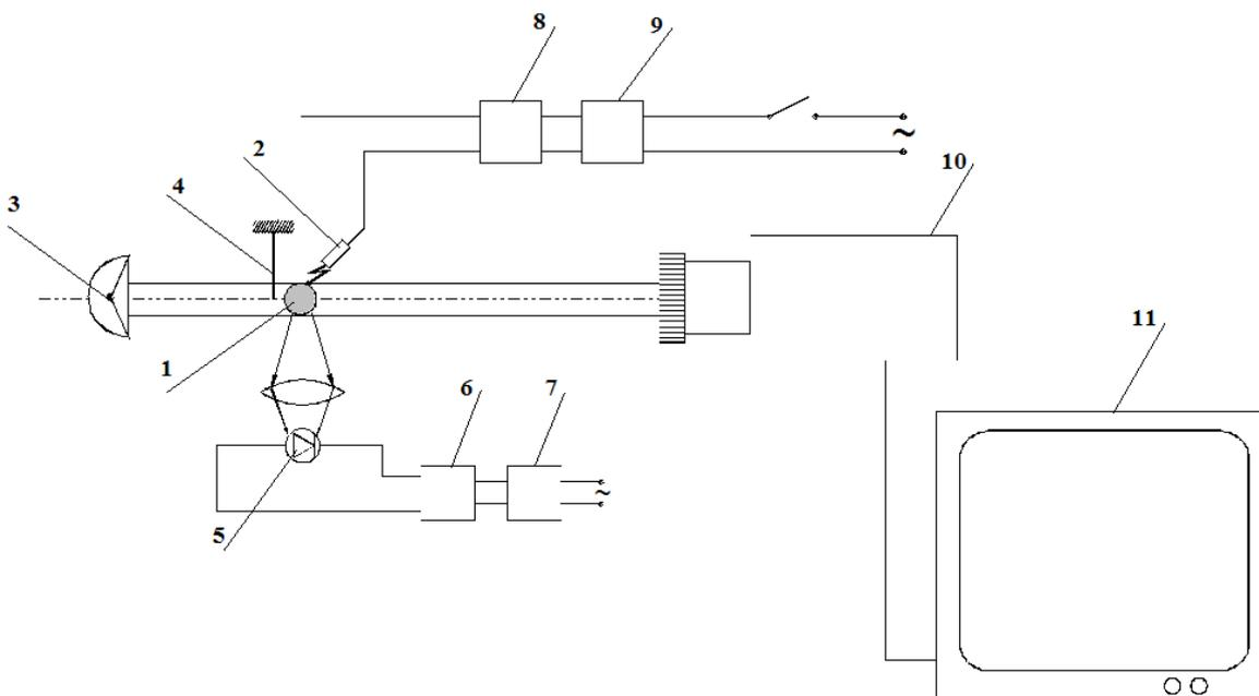
Fig. 1. Scheme for the liquid fuel drop combustion measurement. 1- drop of fuel; 2- spark electrode 3- light source; 4- dimension scale; 5- photodiode; 6- amplifier; 7- electronic timer; 8- spark generator; 9- regulator of the spark transition time; 10- camera with the telephoto lens; 11- monitor
